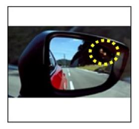
Due to BSM control module production variances, a false detection may occur in some units when the BSM temperature in the control module has not yet reached normal operating temperature. To eliminate this concern, the control logic of the BSM control module has been modified.
