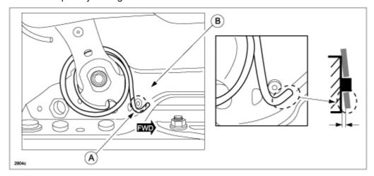
7. Release the rear balance spring (A) hook from the pin (B) using a tool with a hooked end (C) (as shown below) or with needle-nose pliers.
