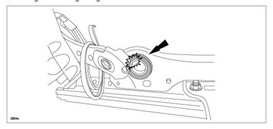
3. Push the link into proper position.
