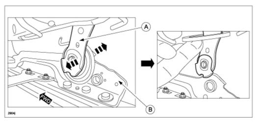
CAUTION: DO NOT damage the bushing during link removal.
