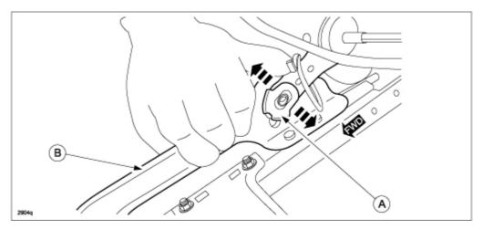
NOTE: Verify that the rear balance spring (A) has been properly positioned around the link (B).
