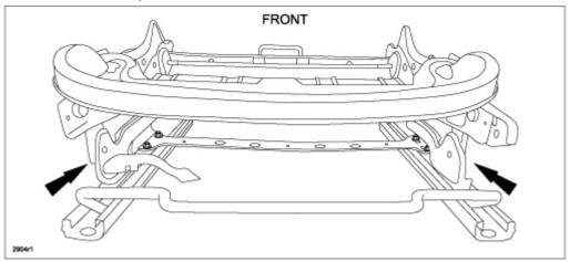
11. Detach the inner link (A) from the slider (B) by gently bending the slider outward and the link inward. **CAUTION: DO NOT** bend the slider too much as it may become deformed and cause improper operation.
