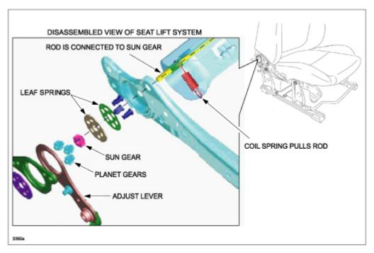
Under normal conditions, the sun and planet gears are held by the coil spring and the leaf springs (as shown below) so the gears do not rotate and change the seat height.
