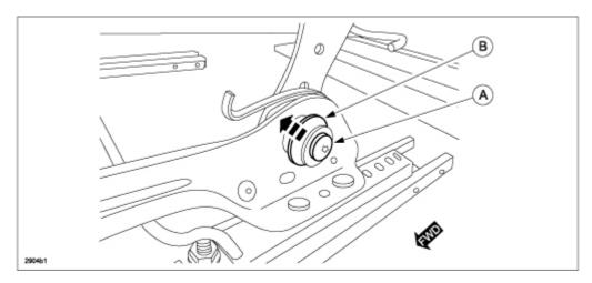
FRONT: Tighten bolt (A) without washer.
