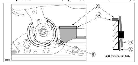
6. Using a flat-blade screwdriver with masking tape on the tip, gently pry the balance spring hook (A) away from the slider surface (B).
