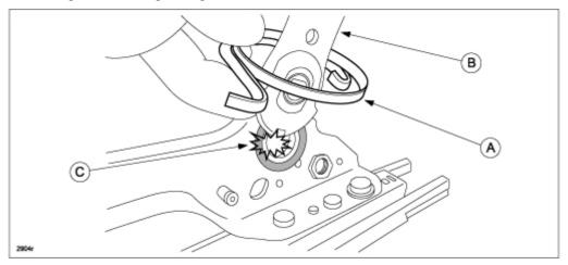
5. Push the link into proper position.
