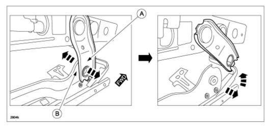
**NOTE:** Depending on specific production date of the vehicle, some CX-5 models may have plastic washers (A) installed between the front link (B) and the slider (C). **ALWAYS BE SURE TO RE-USE THE PLASTIC WASHERS** when installing the new seat adjuster lift unit.
