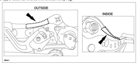
22. After degreasing the upper seat frame area, attach the piece of black tape (from kit) as shown below.
