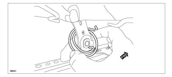
11. OUTER-SIDE: Install the balance spring (A) by hooking the end of the spring into the opening (B).
