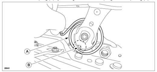
17. Hook the other end of the balance spring around the pin (A) using the hook tool (B) or with needle-nose pliers.
