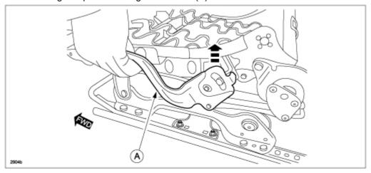
5. Starting with the **REAR** of the seat adjuster unit (as shown below), attach a piece of masking tape onto the inner sides of the left and right sliders to avoid scratch damage during the repair.
