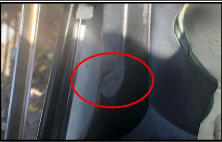
Figure #3: Inspect inner hood for signs of contact.
