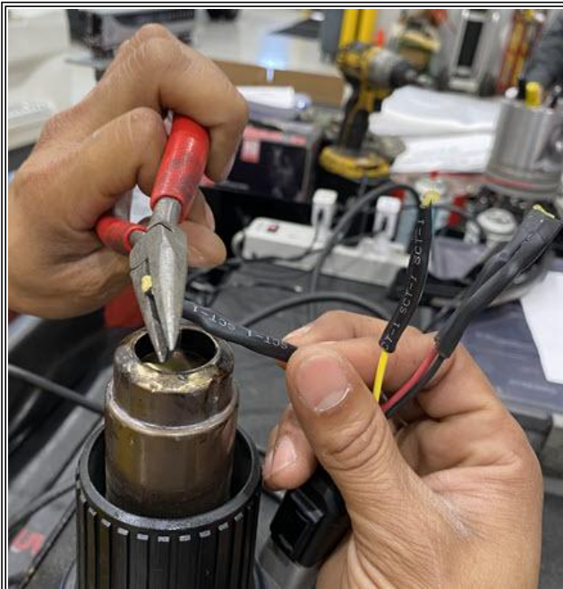
Figure 7: QLS Pigtail Wire Sealing
