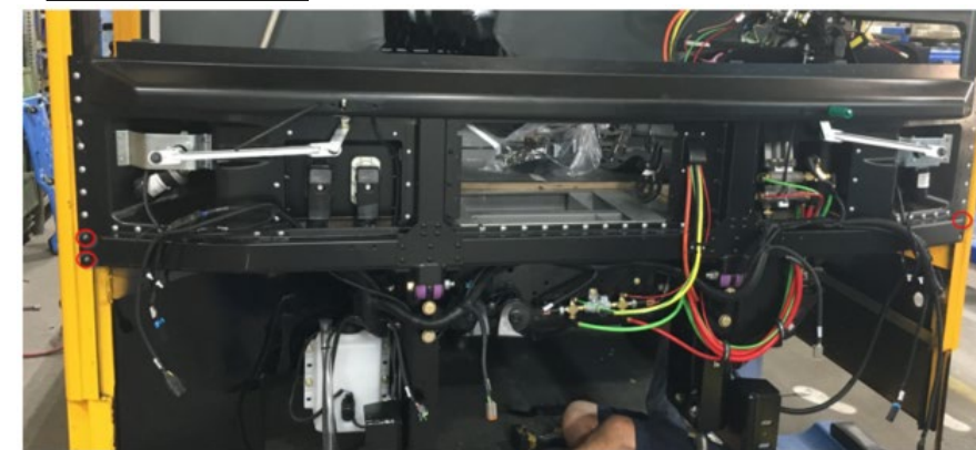
SUBSTITUTED SCREWS & NUTS FOR RIVETS WITH THE EXCEPTION OF CIRCLED AREAS
