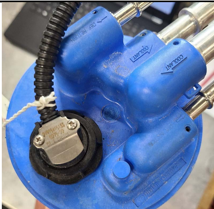
Figure 5: Gen4 Header with Digital Sensor Exterior Closeup
