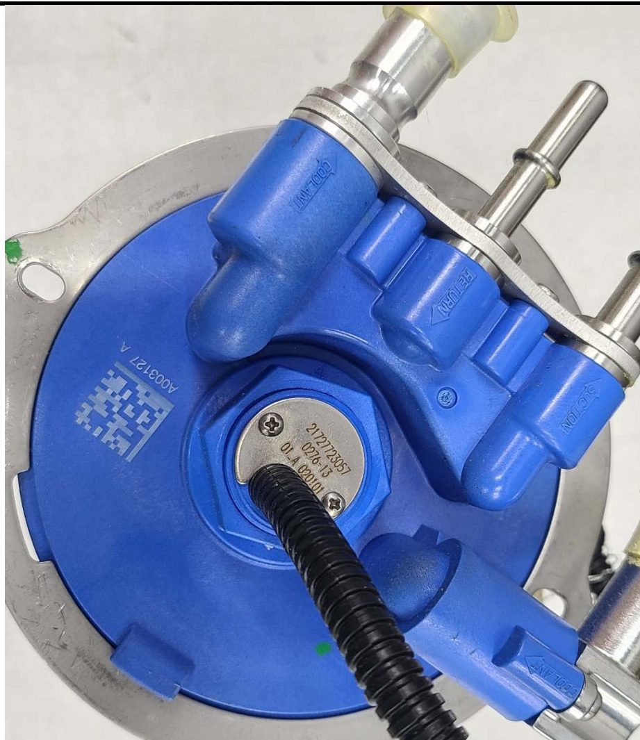
Figure 9: Gen5 Header with Digital Sensor Exterior Closeup
