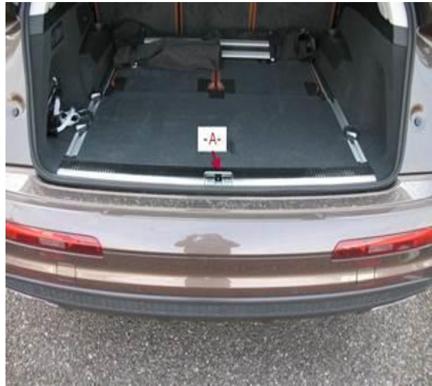
Figure 4. Striker cover opening.
