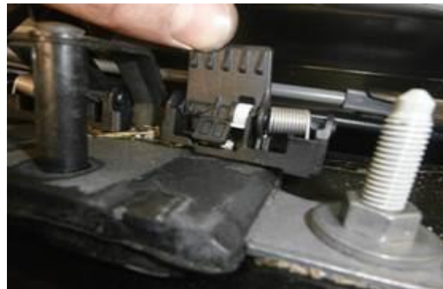
Figure 3. Debris in the rear lid closed sensor.
