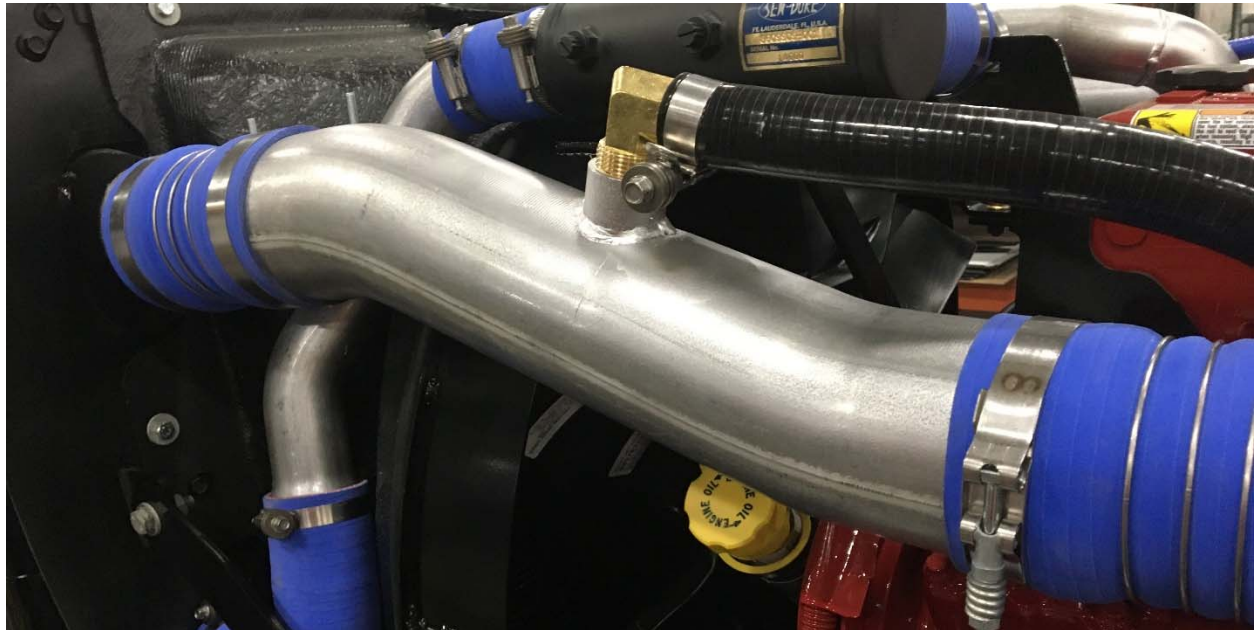
Fig. 2 CAC Cold Pipe and Aire Compressor Intake Hose.
