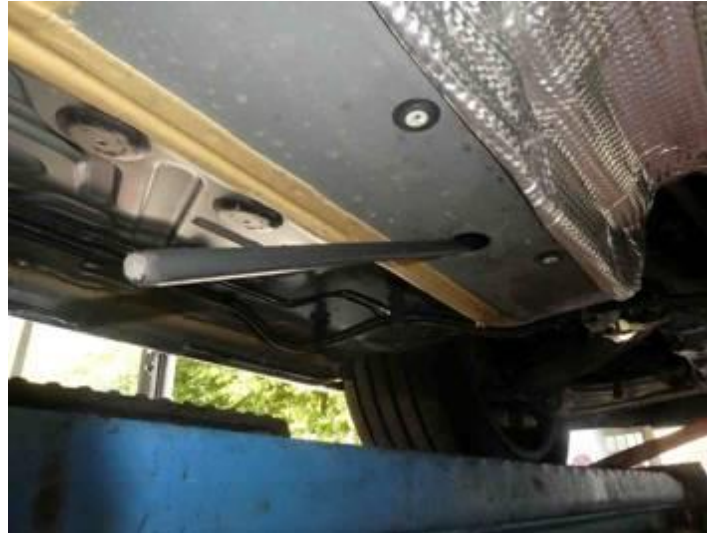
Figure 17. Driving the steel rod into the longitudinal member support.
