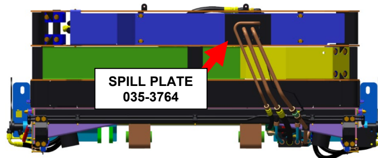
Figure 5. Spill Plate (035-3764) Installation Location
