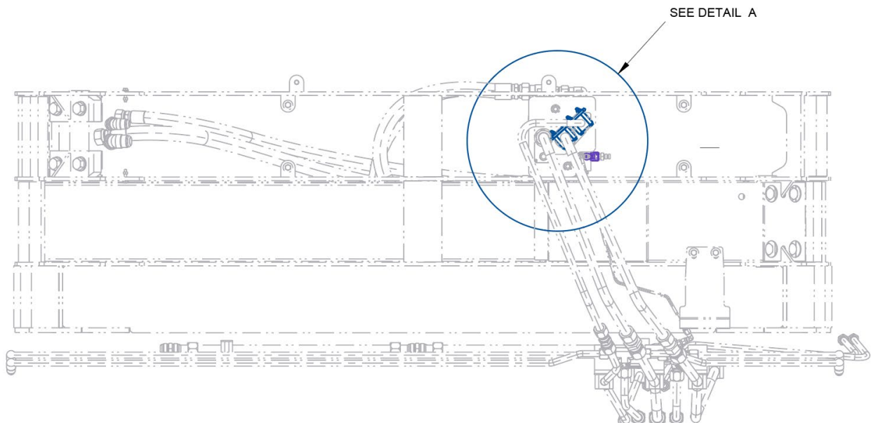
Figure 3. Front Head Tube Support Clamp Installation Location (Thermal Resistant Sleeves not Shown)
