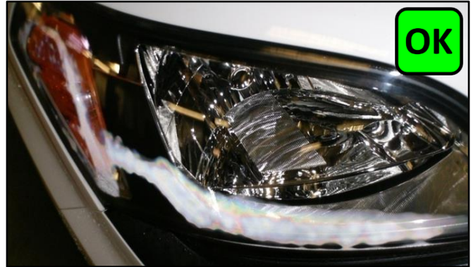
Example of normal condensation in headlamp. No repair or replacement necessary.
