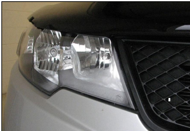
EXAMPLE: Moisture accumulated within the headlamp assembly displays a fogging condition.
