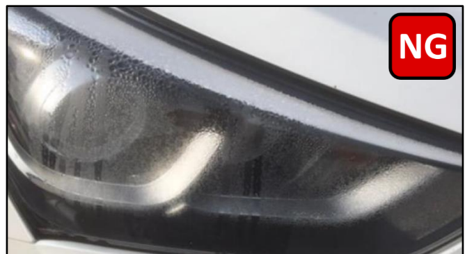
Examples of water leak in headlamp. Water droplets inside of headlamp assembly. Condition should be diagnosed and repaired.
