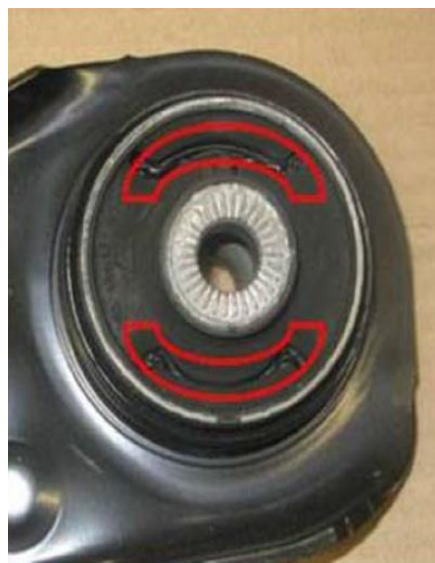
Figure 3. Lithium grease is applied on the red highlighted area only.
