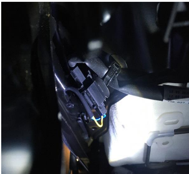
Figure 3. Belt buckle wiring and connector on seat frame.
