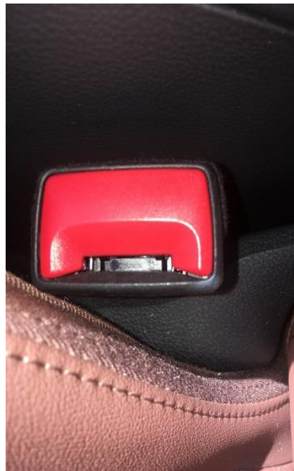
Figure 1. Belt buckle with latching mechanism.
