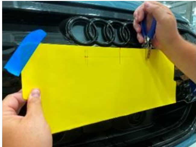
Figure 3. Hole punch through the template.
