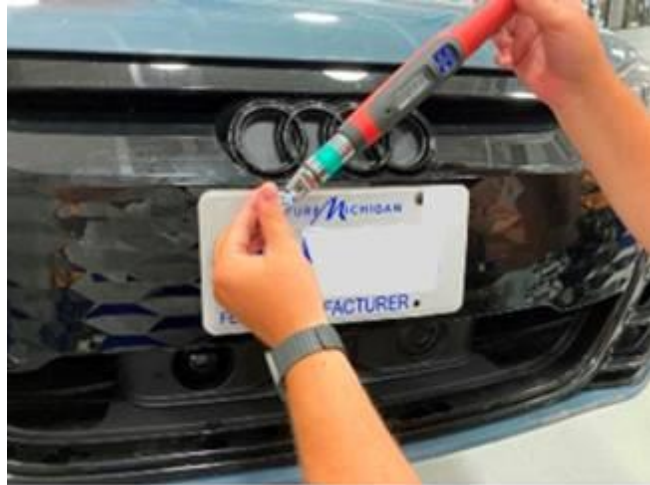
Figure 7. Installation and final torque of the front license plate screws.
