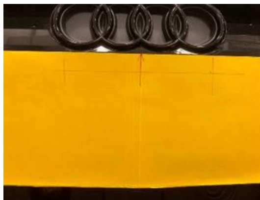
Figure 2. Front license plate mounting hole template.
