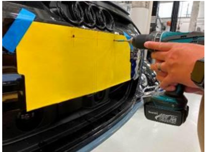
Figure 6. Drilling of the screw holes.
