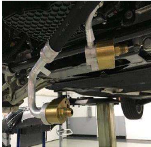
Figure 6. Installation of VAS 6338/3 and 6338/12.
