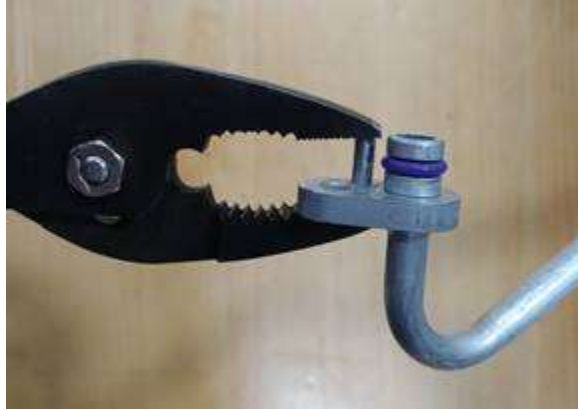
Figure 16. Installation of rear refrigerant line dowel pin.
