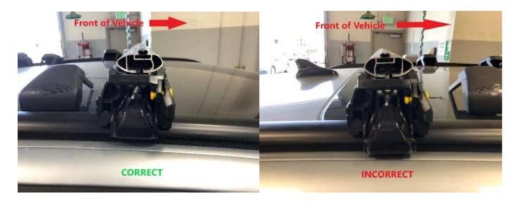
Additionally, ensure the rubber strips (called out in the installation instructions as "cover profile") are installed correctly. Once installed, the cover profile should be almost flush with the top of the carrier bar. It is possible to install the seals upside down. Note the below photos showing correct and incorrect installations of the cover profile.
