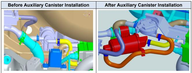
5. After mounting the auxiliary canister, secure auxiliary canister and hoses with cable ties.
