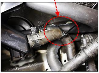
Put a cable tie through an eyelet (H) of the auxiliary canister and tie to the air filter vent hose (I).
