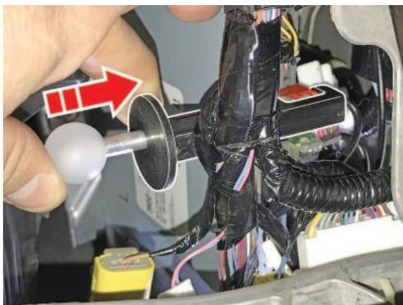
4. While holding down the ball, slide off the connector.
