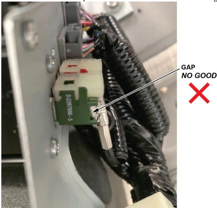
In both examples, the connector is considered damaged, and the wire harness must be replaced. These connectors **are not** repairable.
