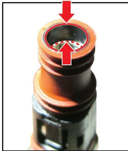
When inserting the wire into the new terminal, make sure you hear a click to ensure it is fully seated.
