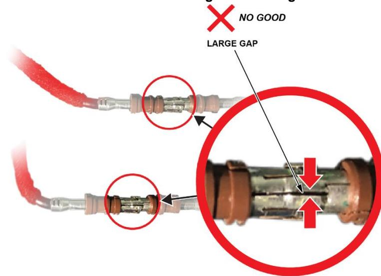
NOTE: The various service bulletin repair procedures available on SIS related to repair MOST-related problems will have you install a new terminal to help avoid terminal spreading. However, it is important to still make sure that the harness wire and connectors are installed back to their original condition.
