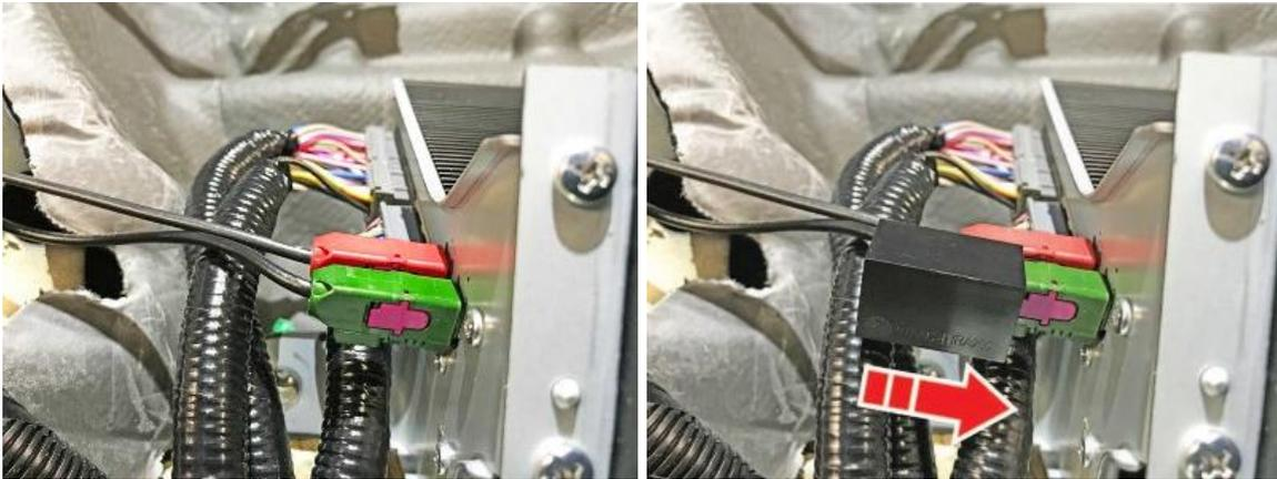
2. Once you feel it click into place, the tool is fully seated. Pull straight back to release the connector.
