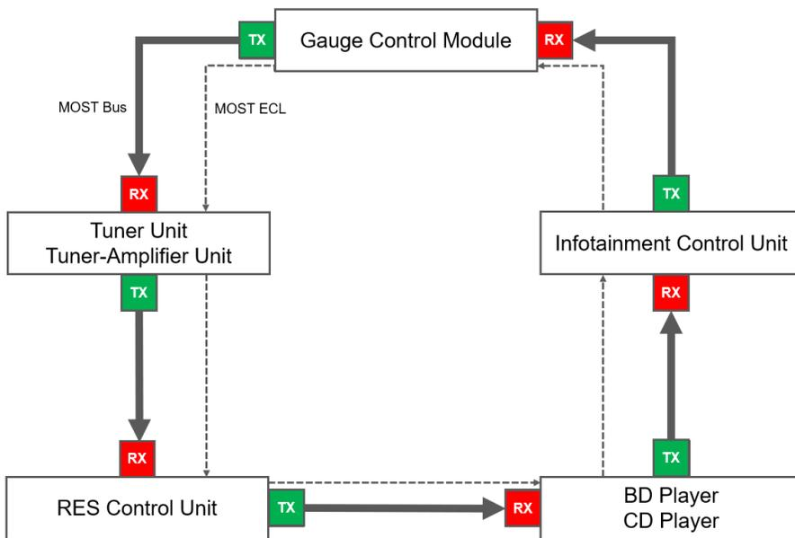
Within the TX and RX connections, there are the TX+ / TX- and the RX+ / RX- terminals. The “+” indicating the information line and the “-” indicating the shielding ground.
