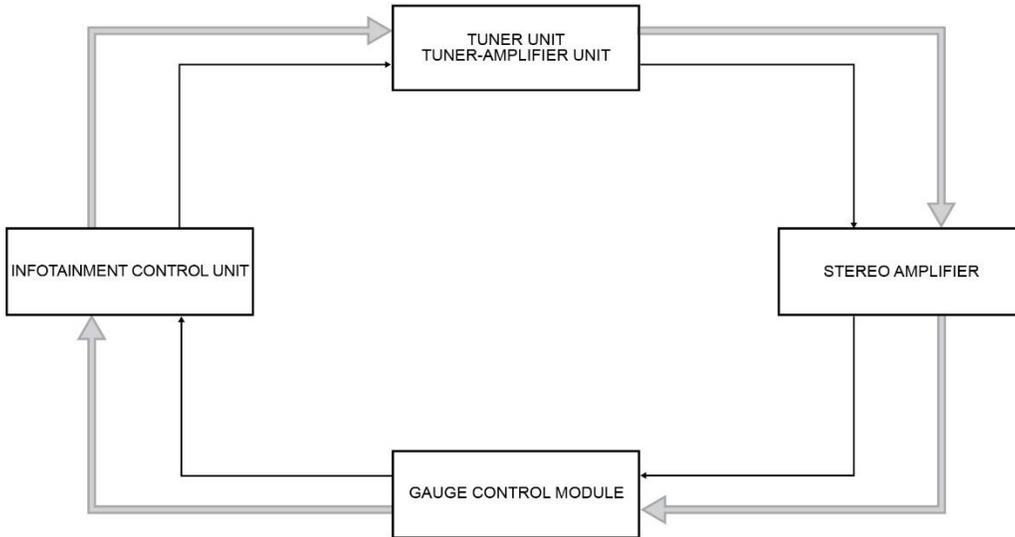
The gauge control module acts as the gateway in the MOST Bus Network. Each control unit on the network has transmitting and receiving coaxial cables and the electronic control line (ECL). The transmitting, known as a TX connector, is green in color, and the receiving, known as a RX connector, is red in color. Any open connections or shorts in the network wiring will cause audio and visual system functions to be inoperative.
