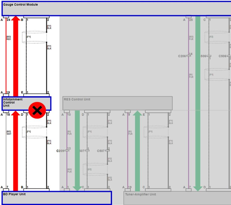
In this next example, the ECL diagnostics results shows the meter, telematics and tuner amplifier reporting problems. After checking the EWD, the telematics (telematic control unit) and the tuner amplifier (tuner-amplifier unit) is not equipped on the vehicle, leaving only the meter (gauge control module).
