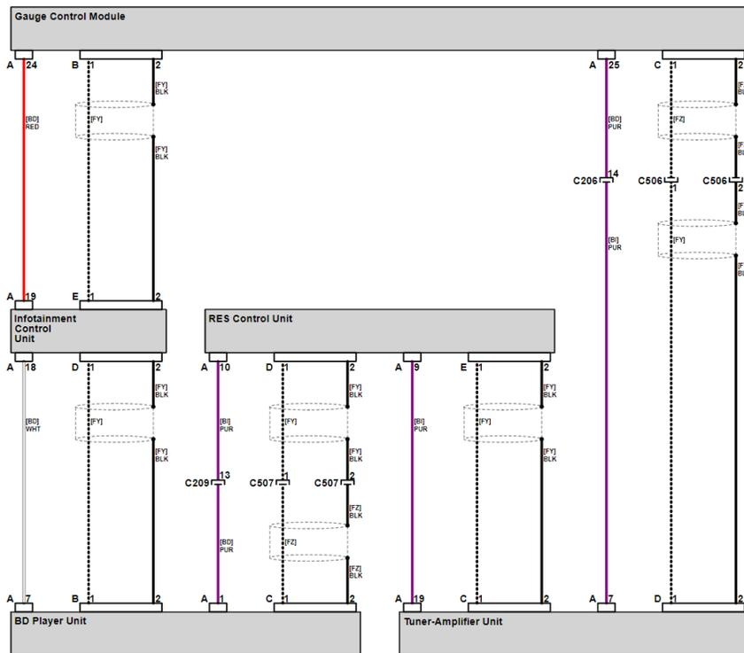
By checking the EWD, the amplifier (stereo amplifier), remote tuner (tuner unit) and telematics (telematics control unit) are not equipped for the model and trim level you are working on and can be ignored. That leaves the meter (gauge control module) and the infotainment (infotainment control unit).
