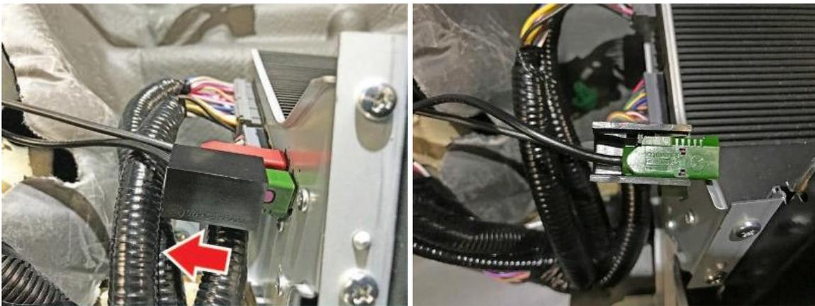
3. Remove the connector from the tool. Rotate the bottom of the connector (opposite the lock tab) out first. This will avoid the lock tab catching on the tool.
