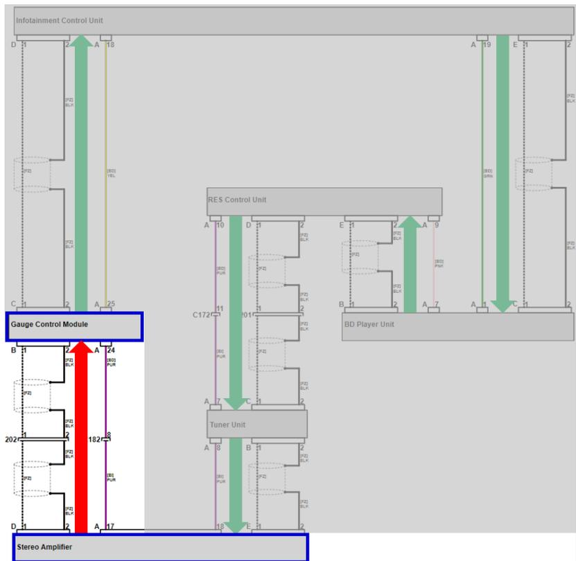
Troubleshooting this circuit revealed a bad connection at inline connector C202.
