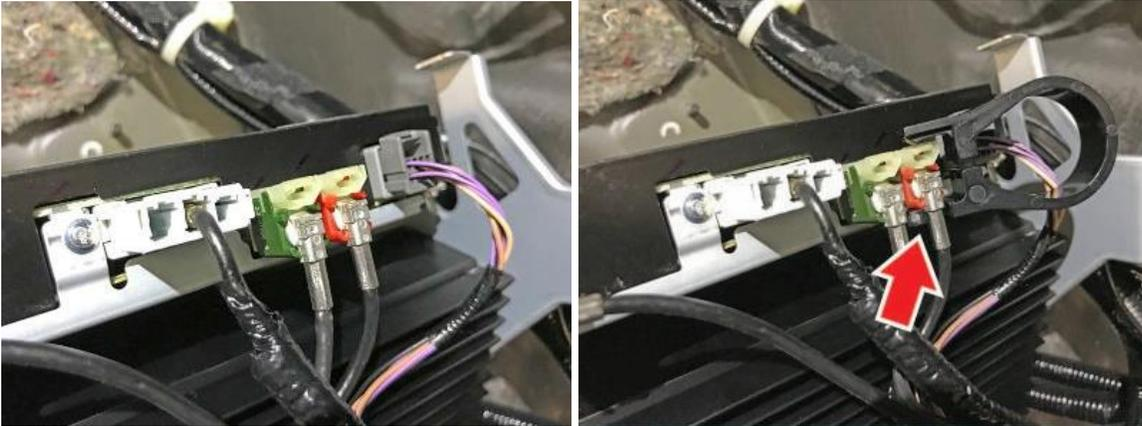
2. Squeeze both sides of the tool to unlock the connector, then pull straight back.
