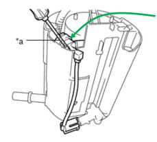
Repair Manual: Using a screwdriver (\*a) with its tip wrapped in protective tape, remove the jet pump from the No. 1 fuel sub-tank.
