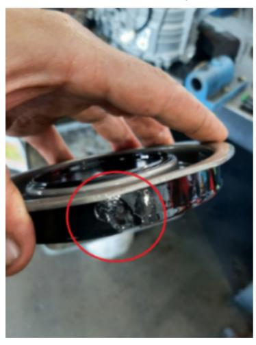
Inspect the edges of the clutch piston for any concerns.
