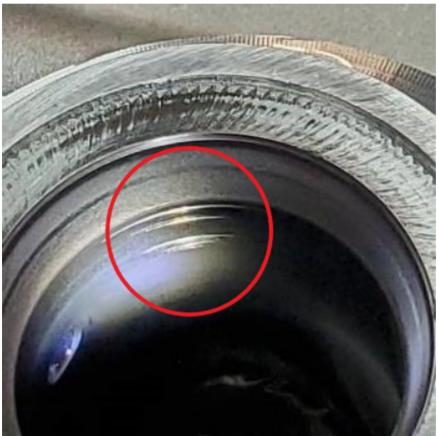
If signs of wear are seen as shown, this indicates the Primary Pulley Bearing has spun in the bore and is allowing the Turbine Shaft to become off center When this happens, it causes a pressure leak.
