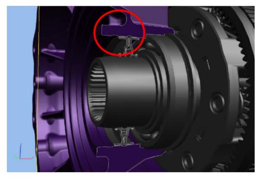
While GM works through the servicing tool strategies, J-45228 (4) can be used to drive the seal in HOWEVER there is no stop at the correct depth. The seal will have to be driven in slowly and seal installed depth checked. Be careful not to drive in to deep or you will need to replace the seal again.
