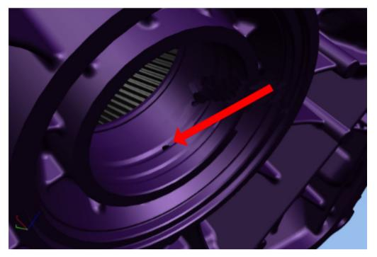
There are 2 design transfer case front case halves and the seals install at different depths between design 1 and 2. To identify design level look for a machined groove where the seal is installed (Red circles below). If there is a defined machined groove in the case then it is a first design case. If there is not a defined groove machined into the case then it is second design.
