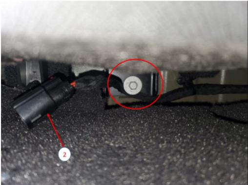
2. Inspect connector X225 for terminal issues/corrosion (3), as shown below. In this scenario, the LIN Bus circuit 4115 was corroded and shorting to other terminals in the connector. If corrosion is found at X225 inspect for a water leak. One known leak location is the A pillar grommet for the door pass through connector not being fully seated.
