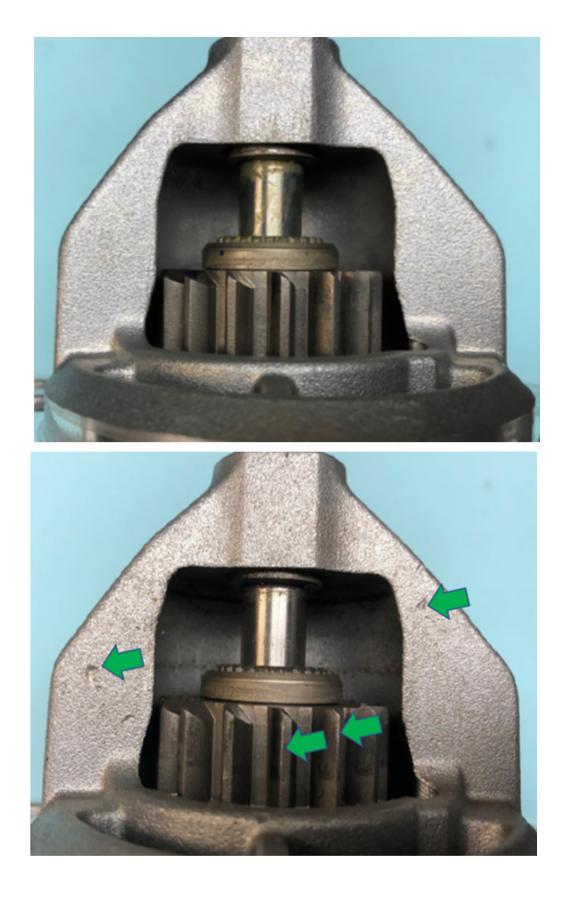
If the starter pinion drive teeth or housing have pieces / chunks missing, replace the starter motor assembly. Examples of starters not to reuse / reinstall
