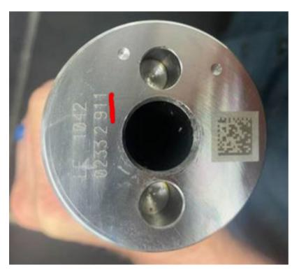
The label below shows the correct camshaft part number 12619823 for L83 the camshaft above should have 823 NOT 911 etched on the end.
