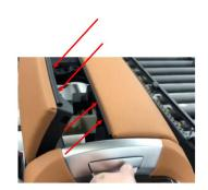
A. The seal between the two halves of the armrest may be sticking. If found, apply lubricant P/N 83 19 9 408 523 to the seal and retest.
