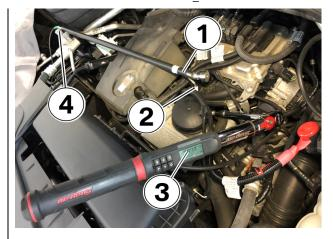
Install the frequency sensor with mounting bolt into the M8 hole (1).
