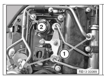
When the high-pressure line connections (1) are released, then the line (2) <u>must</u> be replaced.
