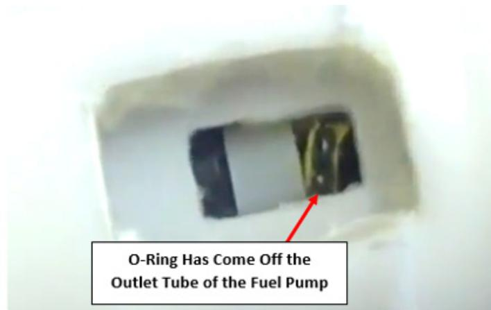
**VERY IMPORTANT REMINDER:** When installing the new fuel pump into the filter housing, it is **CRITICAL** to press the new fuel pump **FIRMLY SQUARELY** and **STRAIGHT** into the filter housing in ONE smooth, continuous motion. Misalignment will prevent the o-ring from seating squarely in the bore and when the hand pressure is released to try again, the o-ring can easily become dislodged from the fuel pump outlet tube resulting in the mis-alignment shown above and in the illustrations below.
