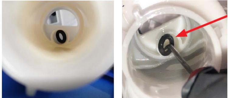
Both the illustration and picture below show the proper configuration of the fuel pump, bushing and o-ring prior to reassembly. The new o-ring is positioned for proper sealing on top of the bushing.
