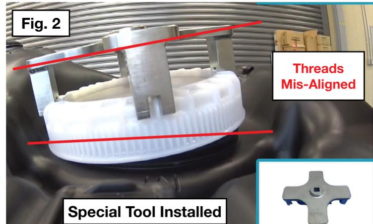
**Figs. 3 & 4** show the Special Tool is installed onto the Ring Nut then, a firm, sharp, **straight downward** force being applied to the tool to “jump” the threads resulting in proper alignment and start to a normal, successful tightening procedure.
