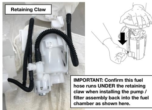
**IMPORTANT:** Confirm this fuel hose runs UNDER the retaining claw when installing the pump / filter assembly back into the fuel chamber as shown here.
