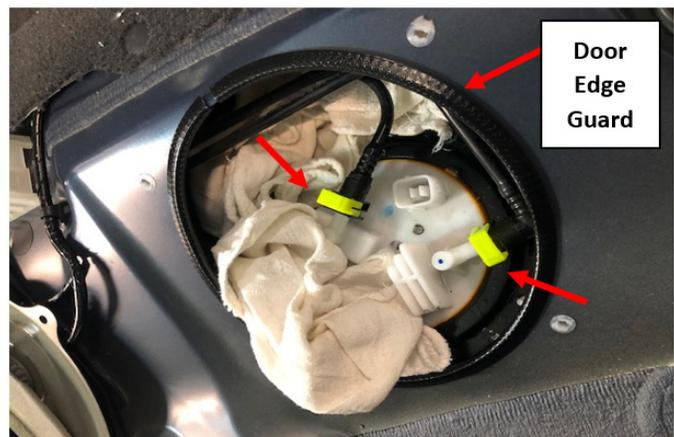
On Legacy and Outback models, use a small container or magnetic dish to keep all the retaining ring nuts together while the pump assembly is removed.
