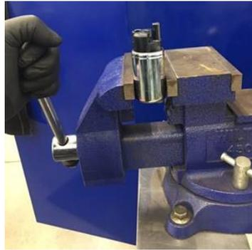
**IMPORTANT:** Remove the o-ring and spacer from the original fuel pump. The spacer is reused. Put the removed pump in a vise and crush it as shown here to eliminate any chance of it being reused.
