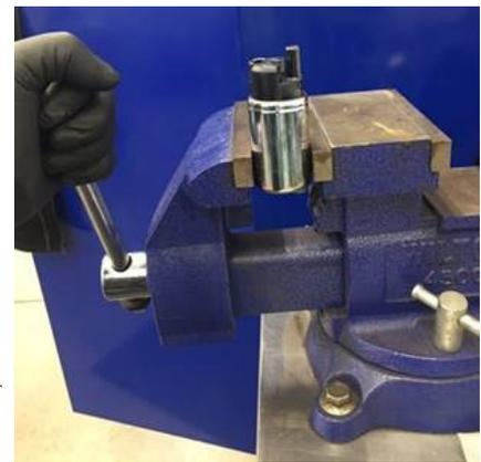
**STOP HERE DO NOT** remove the pressure regulator or otherwise go any further with disassembly of the fuel pump assembly.
