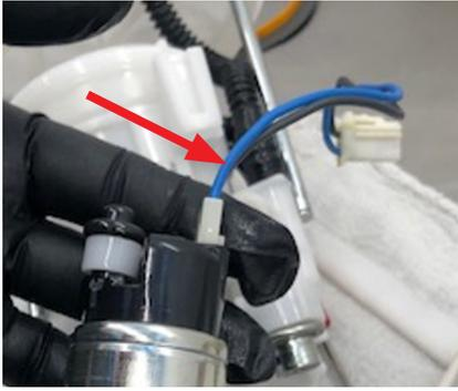
For this recall, the 2-wire (Blue / Black) fuel pump wiring harness indicated as 1-time use in the Service Manual is reused but, should be inspected for damage or any evidence of overheating (discoloration of connectors, etc.). **IMPORTANT:** If any damage e.g. distorted or melting plastic connectors, overheated wiring or terminals is identified, the harness **MUST** be replaced. It easily unplugs from the fuel pump.
