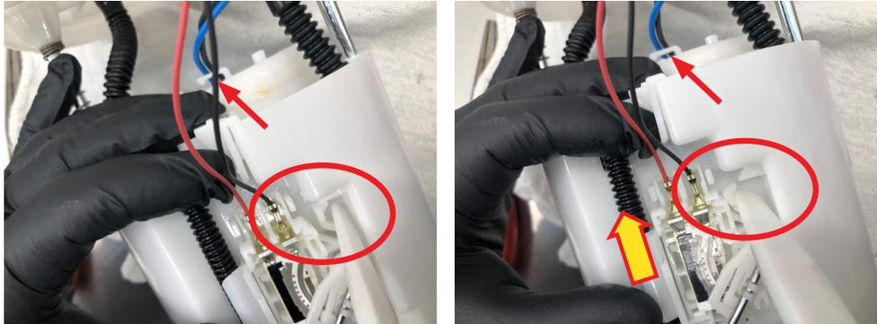
7. **CAREFULLY** disconnect both the fuel pump and fuel sending unit harness connectors and remove the wiring from the retaining clips. Note the wire routing prior to disassembly for reference during reassembly.
