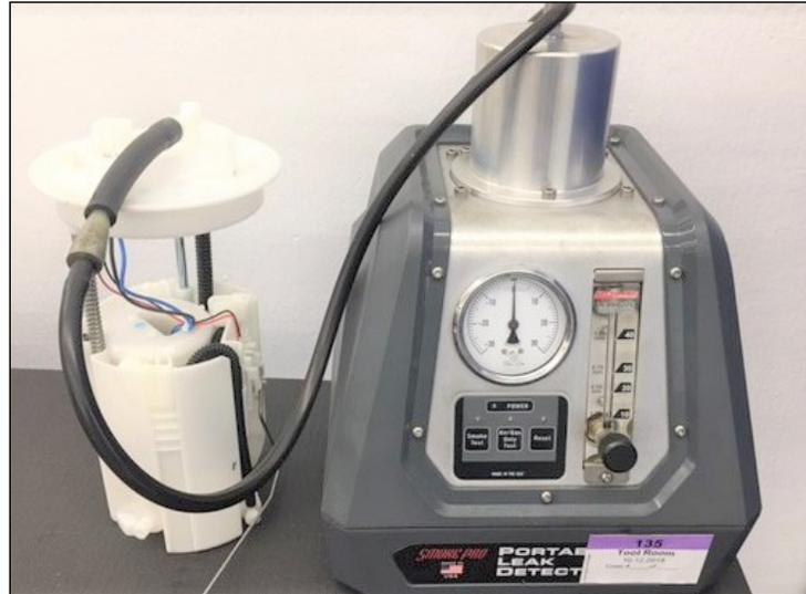
9. **IMPORTANT:** Make sure all the sealing surfaces are free from fuel or foreign matter before reinstalling the fuel pump assembly.
