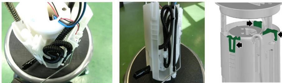
**ALWAYS** inspect closely for any seepage or leaks around ALL fuel delivery tube connections removed as part of this repair (including those under the hood if fuel was drained) and around the ring nut.
