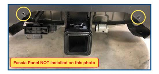
STEP 5) Install the clips #909140062 into the drilled holes. Confirm the fascia maintains minimal gaps and is secured properly to the bumper cover as shown below to complete the procedure.
