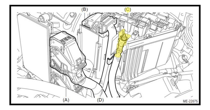
**STEP 4)** Using the SSM, check the CID to determine if the ECM requires reprogramming. Compare the current CID to the "**GOOD**" CID numbers supplied in the table below.
