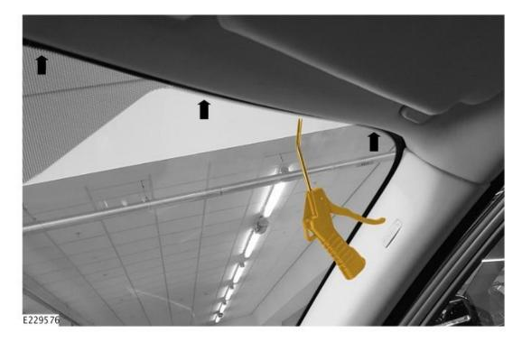
Using an air blower, blow compressed air around the inside edge of the windshield, as shown in the illustration.
