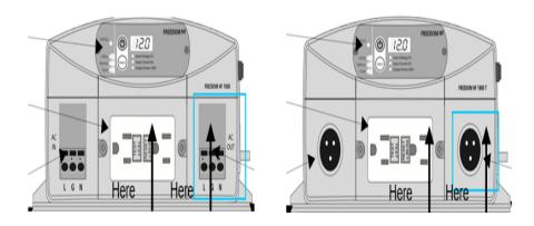
If there is voltage on the hardwire contacts but none on the **GFCI:** The problem is a tripped GFCI, faulty GFCI, or wiring problem to the GFCI.
