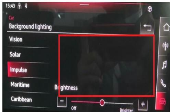
Figure 1. Picture is missing in the interior lighting menu.
