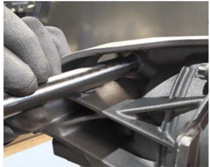
Figure 5. Installing sealing cap
