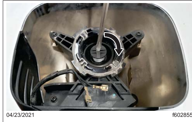
Fig. 2, Placing and Securing the Spring-Loaded Locking Pin
