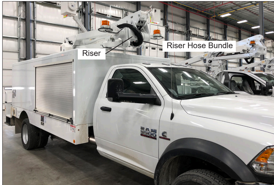
Figure 1 — Hose Bundle at Riser
