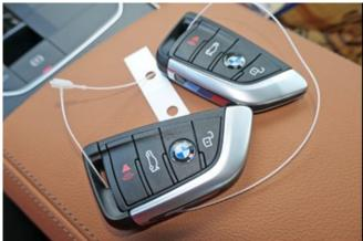
Vehicles were delivered with the wrong radio remote control (without motion sensor) which decreases the theft-proofing against range extenders.
