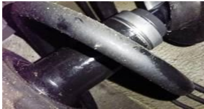
Figure 1. DRC shock absorber with clear oil loss.
