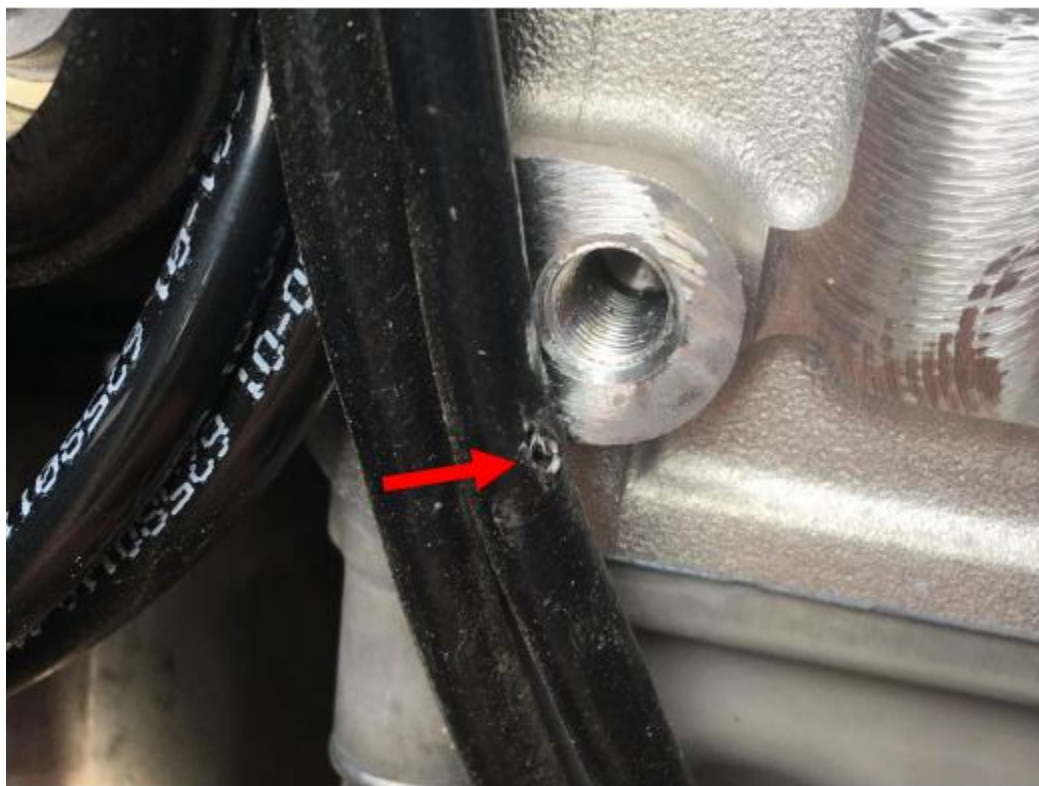
Figure 2: K69 Oxygen sensor bank 2 - damage of the lines, wiring harness at the bracket for engine spoiler
