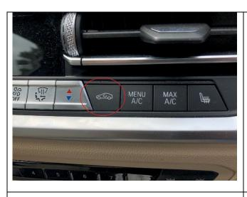
1. Deactivate the air recirculation function by pressing the recirculation button on the climate control panel (Fresh Air mode, circled), LED off.
