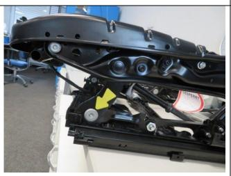
3. Replace the front outer bolt with part number 52 10 5 A13 770.
