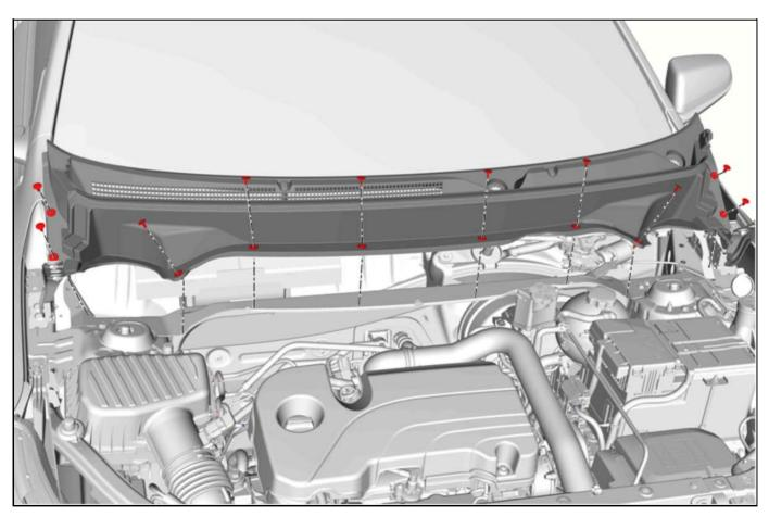
3. Re-install the air inlet panel & wiper arms, making sure the seal from panel on the windshield is flat and touching the glass. No raised areas should be seen. Refer to *Air Inlet Grille Panel Replacement*, in SI.
