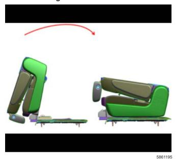
1. With the rear seat in fold and tumble position, return the seat to it's latched position under normal application force (DO NOT SLAM SEAT).
