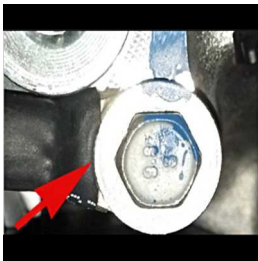
Figure 1: Shown in the picture above is the ground bolt to the engine block (passenger side).
