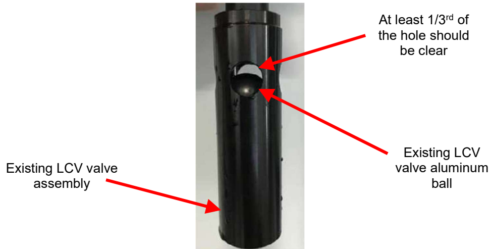
Figure 7: Example of Correct Aluminum Ball Height and Vent Hole Space
