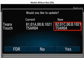
NOTE: If the screen does not appear, the software may not have correctly downloaded onto the USB flash drive. Try to download the software again.
