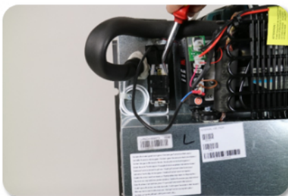
Disconnect the wires from the thermostat
