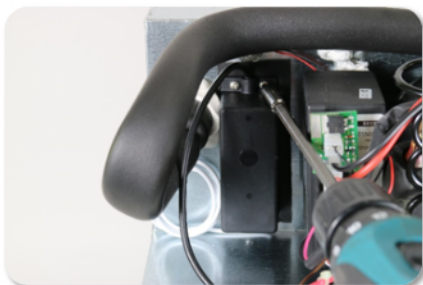
Unscrew the thermostat box (3 screws)
