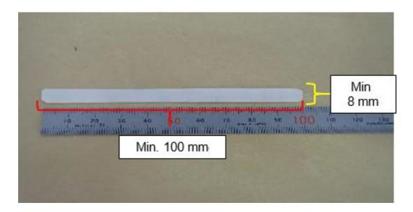
b. Cut off all corners of the protector tape to prevent it from peeling off.
