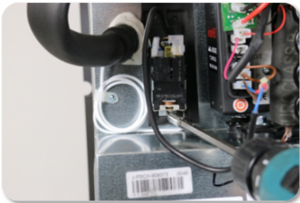
Unscrew the thermostat and the thermostat sensor holder (3 screws)
