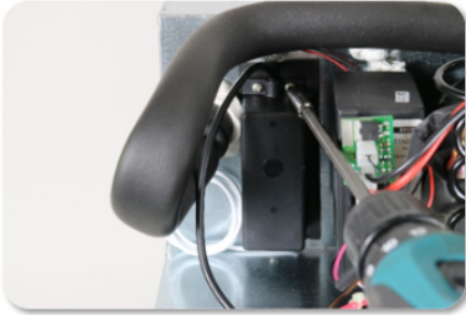
Unscrew the thermostat box (3 screws)
