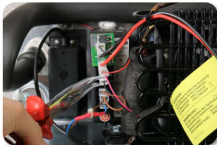
Disconnect the fan wires (pink and black wires) from + and F connector of the ECU
