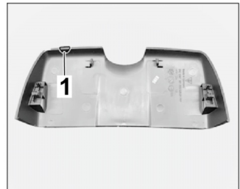
File down the area around the line output
