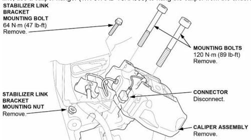
2. With the parking brake released, disconnect the electronic parking brake actuator connector.
