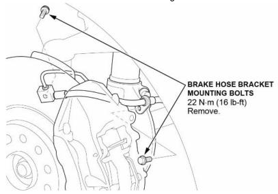
2. Disconnect the connector and remove the caliper assembly without disconnecting the brake line from the caliper body.
