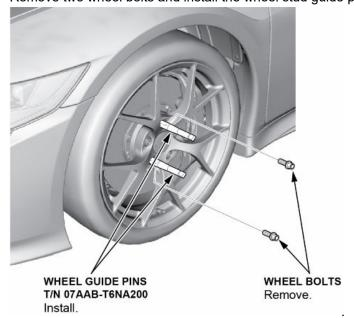
4. Remove the remaining wheel bolts, remove the wheel, then remove the wheel stud guide pins.
