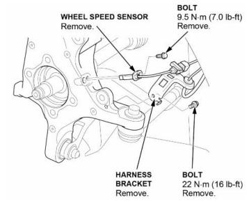
5. Remove the electronic parking brake caliper.
