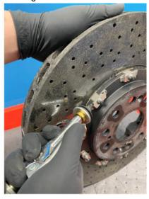
2. Using an approved brake cleaner, clean the face of the disc, and apply generously to the bobbin area.
